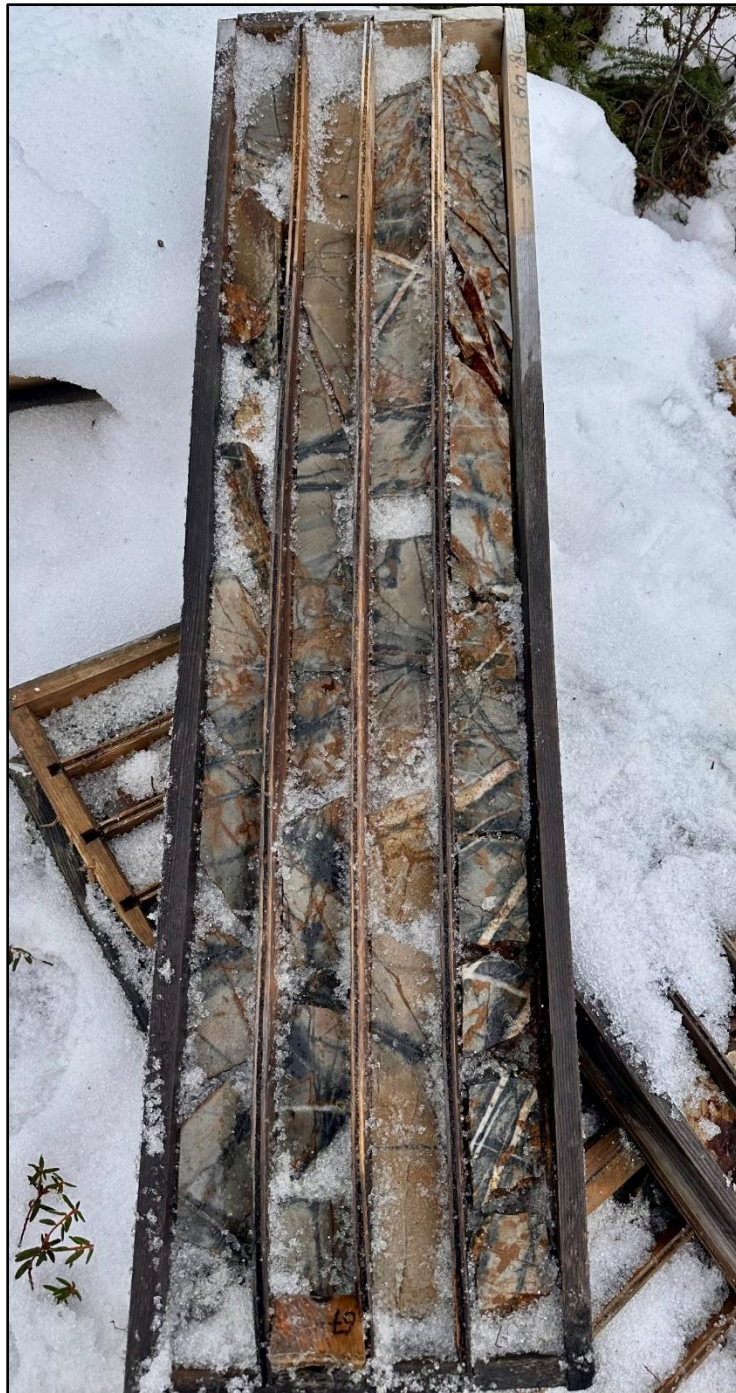
Figure 12: Drill hole core box KZ-08-08 at approximately 62.5 to 67.5 m depth, showing stockwork quartz veins with tourmaline and sericite halos coated with limonite
